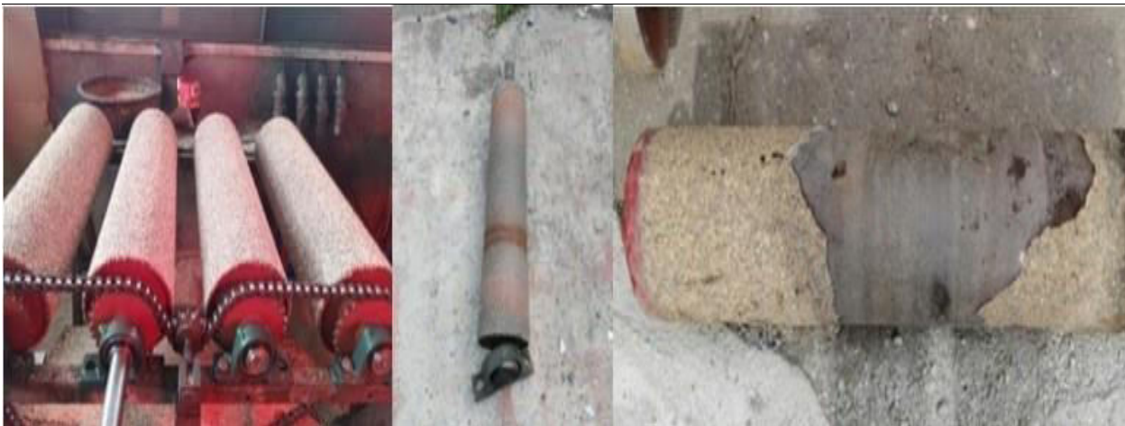
Fig. 1 Presentation of the composite structure of a brake cylinder; a - current technology; b - defects caused by premature wear; c - exfoliation of composite material layers.
